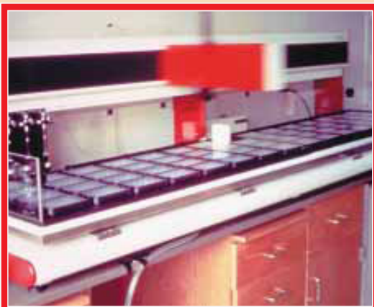
This robot helps prepare tests for mapping DNA markers, filling pipettes with tiny volumes of liquids.
